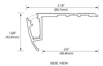
The **4810** Topline Series Step Lighting is an aluminum stair profile with LED tread illumination with single or RGB color options. Perfect for theater applications this profile offers an optional lighted aisle marker with number, letter or symbol.
