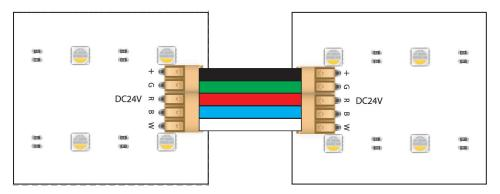
Sheet to Sheet Jumper Linking - Recommended Wire Gauge: 22AWG (Standard Core)
